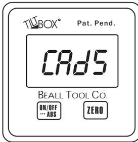
7) Turn the box another 90 degrees clockwise; press the ZERO button-the screen will read CAD5. After 1 second the display will read 0.00-this completes the calibration.
