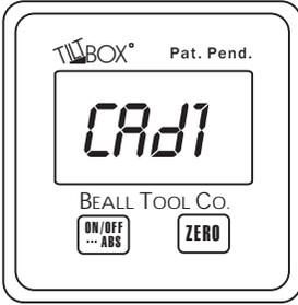
3) Press the ZERO button; the screen will display CAD1.
