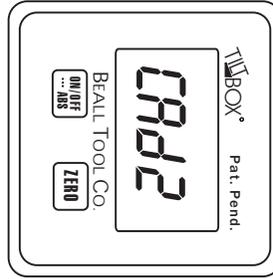
4) Turn the box 90 degrees clockwise. allow 3-4 seconds for the Tilt Box to settle then press the ZERO button-the screen will read CAD2.
